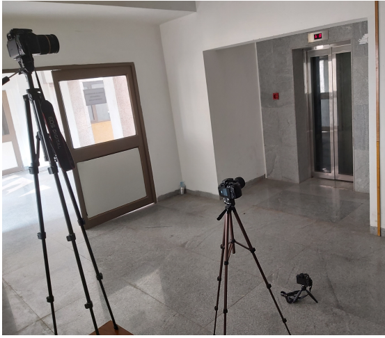
Fig. 6. Experimental setup - three cameras to read the ball height and the base collision; vertical metre scale fixed along the wall
